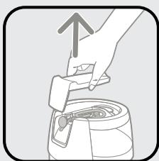
Tear off the BeerTender Keg lid and dispose of it. Beneath this cover is a tap which is connected to the BeerTender keg by a slender tube which guarantees quality and hygiene.
