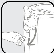
After installing the BeerTender appliance you must clean the dispensing spout; this is the only part of the appliance that will come into contact with the beer.
