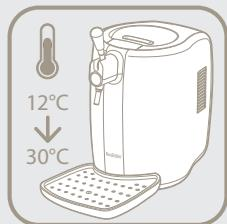
The temperature of the room must be between 12°C and 30°C. Set the drip tray and grate in place at the front of the appliance. Make sure the drip tray is properly fitted and positioned.
