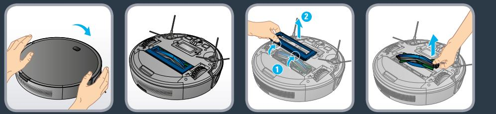
**EN** Clean the brush of the robot once a week. To do that turn the robot upside down. To remove the brush, open the brush guard by pushing the 2 snap latches and pull it up. Then pull out the brush from the robot.
