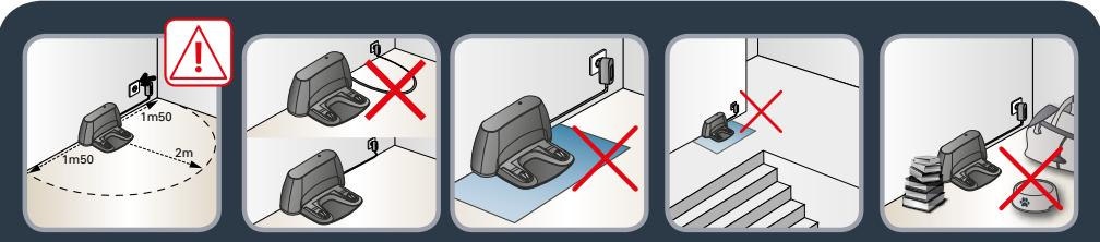
**EN** To place the docking station, make sure there is an empty area of 1.5m on each side and 2m in front of the docking station. Do not install the docking station near stairs. The cable must be tight. Always place the docking station on hard floor. Do not place the docking station on carpet.
