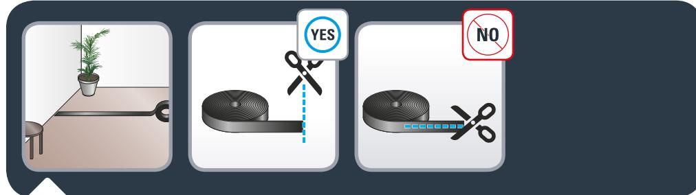
**EN** Should you like to restrict access of the robot to some areas, use the magnetic stripe. Put the magnetic stripe on the floor to mark a no-go zone for the robot.
