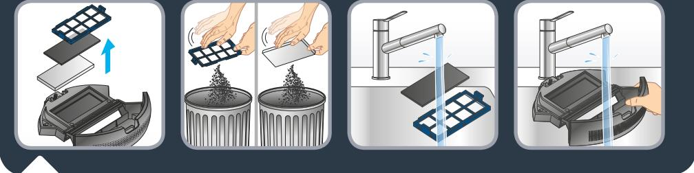
**EN** Clean the filter cover and the filter by tapping the back, holding it above a waste bin. Wash the foam filter, the filter cover and the dust catcher in clean water. Do not wet the fine dust filter (white filter). The filters must be cleaned at least once a week.
