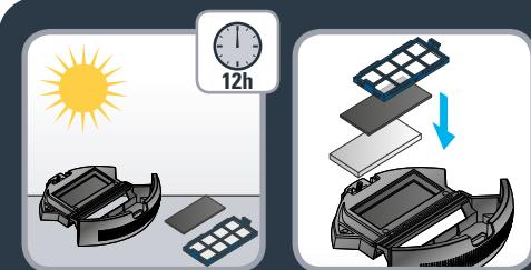
**EN** Let all parts dry approximately 12 hours. Do not use wet filter or dust container. When dry put the filters back in the dust container.
