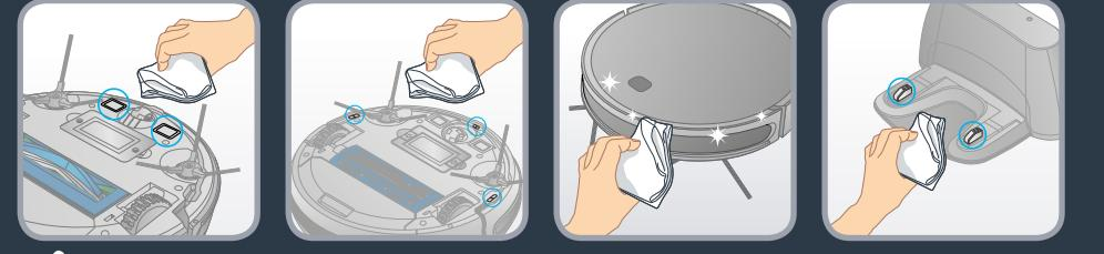
**EN** Once a week, clean the following parts with a clean, dry cloth: the robot's charge plates, fall sensors, distance sensor, the docking station's charge plates and the robot's front wheel.
