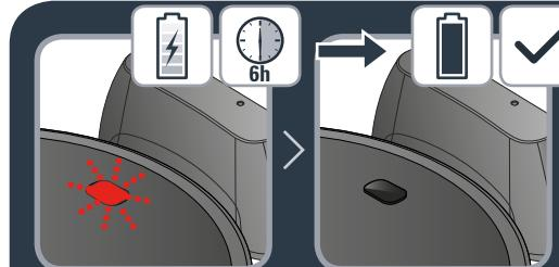
**EN** When the on/off button blinks the robot is charging. Once the on / off button stops blinking it is fully charged (6h for the battery to be fully charged).
