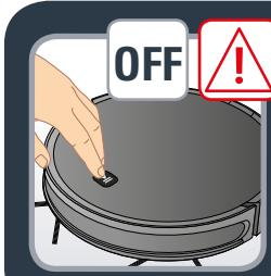
**EN** Attention: Before touching sensitive parts of the robot make sure it is turned off by pressing the on / off button 3 seconds.
