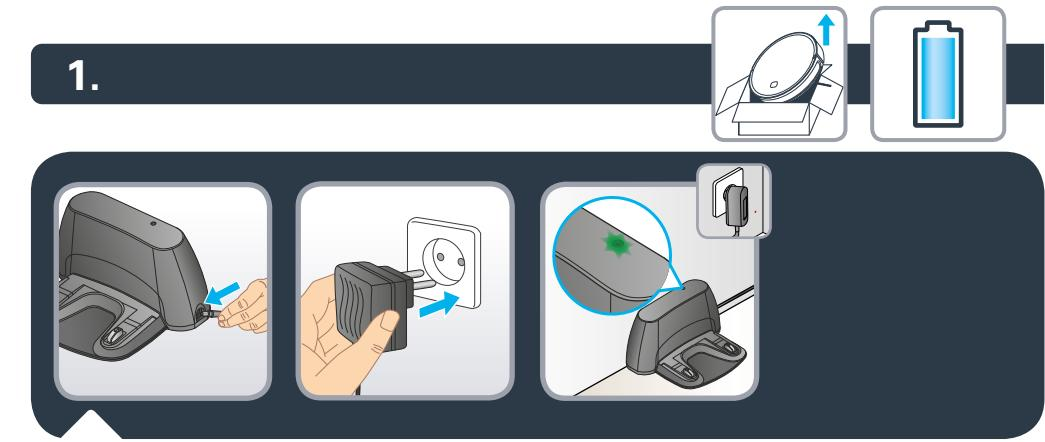
**EN** Plug the adaptor to the power jack on the side of the base. Only use the charger provided with the robot: do not use universal chargers.
