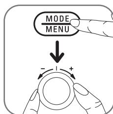
To choose the mode of cooking, press **MODE MENU** key. Select the mode of cooking by turning the rotating knob (1e).
