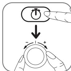
Press **Ø** key. Set the duration of cooking by turning the selector until the desired time. The digital display tells you the time in hours and minutes (e.g.: 0:45).
