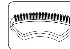
The fabric brush opens the weave of the fabric for better steam penetration.
