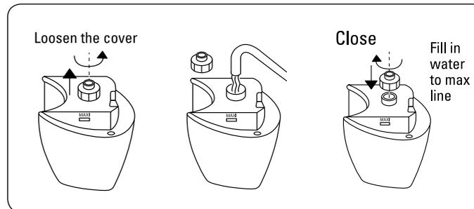
from main unit by releasing container lock and pulling up. Unscrew the cover and fill. Do not fill above the max line on the water tank. Water container capacity is 3.4 quarts.
