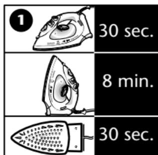
If the iron is not moved while it is plugged in, an internal safety switch will turn it off. It will turn off in 8 minutes if left vertically or in 30 seconds if left on its soleplate or tipped over. A red flashing light indicates that the auto-off has been activated. To switch the iron on again, move the iron or gently shake it. Wait until iron is fully reheated before use.
